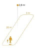
Possible mounting height: 2,50 m - 3,50 m Orange: radial and tangential
